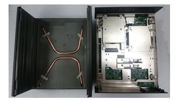
2. Lift up the body of unit. Make sure that both front and rear panels are in the chassis groves and assemble the body on to chassis firmly.
