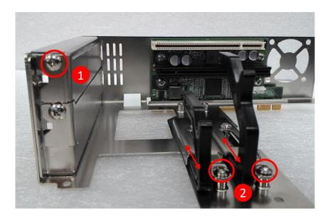
5. (1) Insert a PCI(e) add-on card to the slot. (2) Fasten the screw to secure it (3) Push the card retainer forward to against the edge of the add-on card. (4) Tighten the screw to fix the card retainer.
