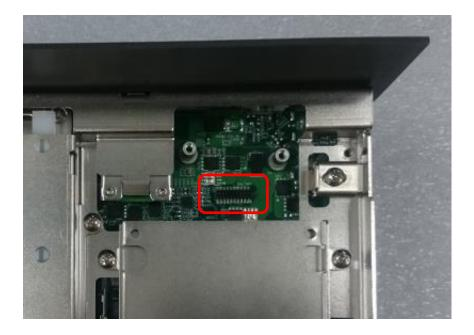
2. Insert the power ignition module carefully into the connector on main board. Fasten 2 screws to fix it.
