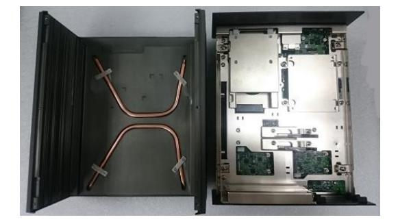
5. Lift up the unit vertically by holding the front and rear panel.
