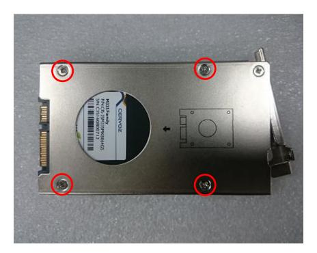
5. Align the HDD bracket with the entrance of HDD bay. Holding the rotating arm and insert the HDD bracket until the connector of HDD contact the SATA connector firmly.
