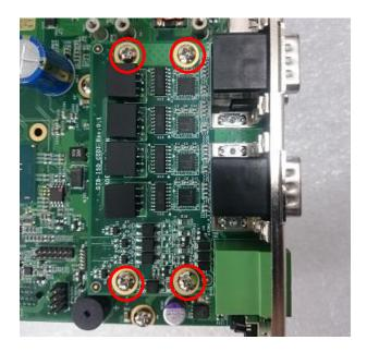
4. Fasten the 8 D-Sub jack screws as marked on photo.
