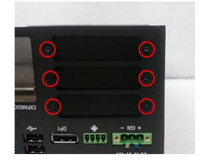
1. Unscrew 6 screws to remove 3 I/O brackets from rear panel.
