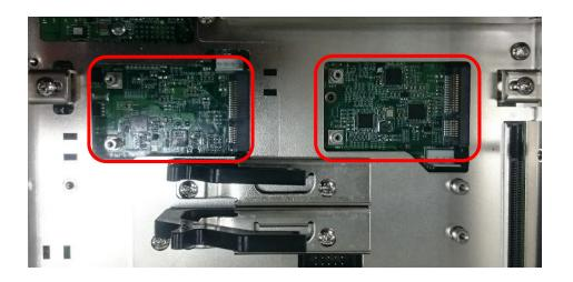
2. Tilt the Mini-PCIe module at a 45 degree angle and insert it to the slot until the gold-pated connector of module contacted firmly with the slot.
