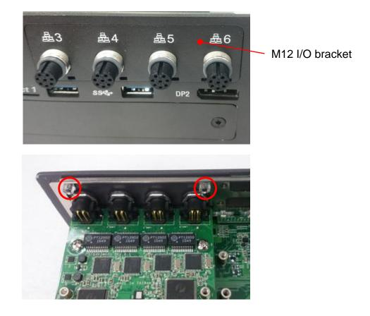
7.Fasten the 4 ring nuts onto M12 jacks.
