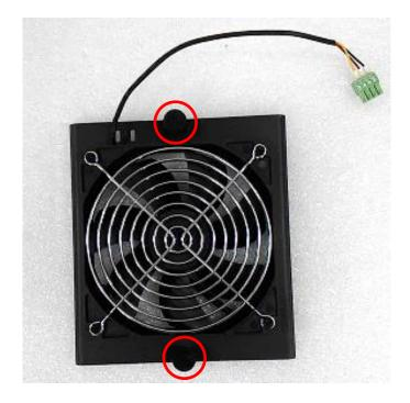
2. Slide the FAN into the middle groove of chassis as illustrated. Tighten the 2 screws to fix it onto chassis.
