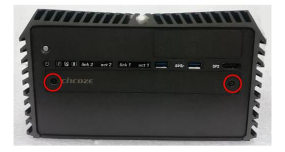
2. Locate the removable HDD bay and loosen the screw.
