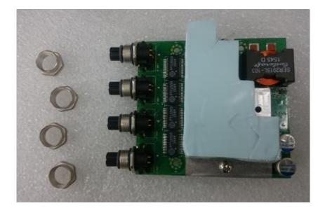
4. (1) Penetrate M12 jack of the module through the I/O hole. (2) Insert the LAN module carefully into the CMI connector on main board as illustrated.
