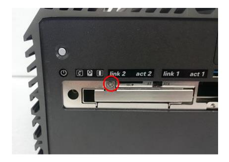
3. Move the rotating arm out and pull the HDD bracket out.
