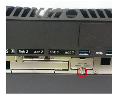
2. Pull out the CMOS battery bracket with assistance of a tweezer.
