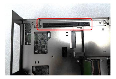
7. Install the module assembled in step 4 into the riser card slot, and fasten the 4 screws to secure it.
