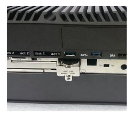
3. Insert a CMOS battery in the battery slot.
