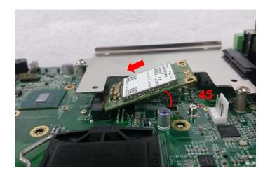
4. Press down the module and fasten two screws to secure the module.
