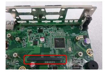
3. Insert the CMI module carefully into the CMI connector on main board. Fix it with 4 screws.
