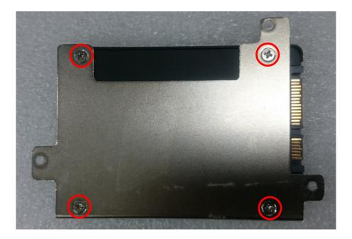
3. Turn over the HDD bracket. Connect the HDD bracket to the SATA connector and fasten the 3 screws .
