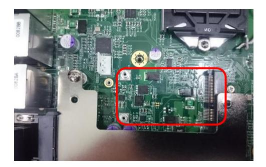
2. Use provided two screws fasten the half size module and adapter bracket together as shown in Fig (a) below.
