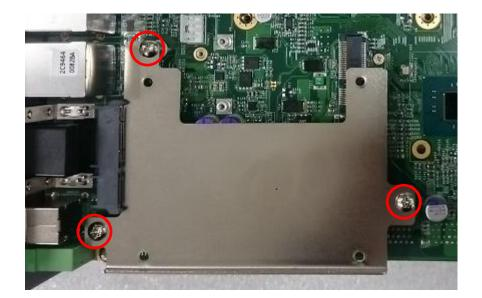
2. Make the PCB side of the HDD face up, place the HDD bracket on it. Ensure the direction of bracket is correct and use 4 provided screws to assemble HDD and HDD bracket together.
