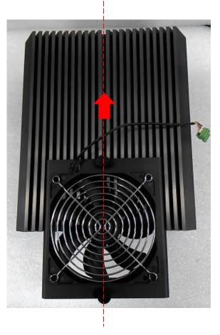
3. Move the fan to the center of chassis. Tighten the 2 screws marked on photo to secure it.
