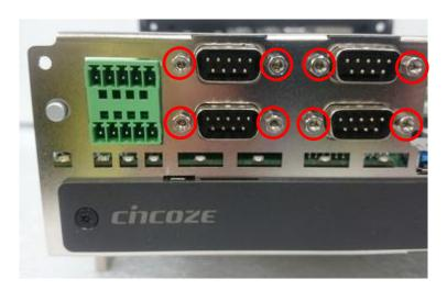
5. Exchange with the front bezel of low speed CMI module as illustrated.
