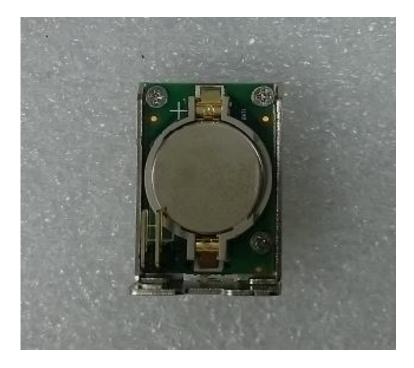
4. Insert the battery bracket firmly and fasten the screw.
