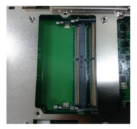
3. Tilt the SO-DIMM module at a 45 degree angle and insert it to SO-DIMM socket until the gold-pated connector of module contacted firmly with the socket.
