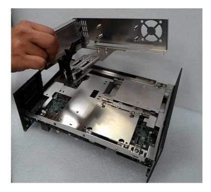
3. Assemble the riser card with extension bracket together and fasten with the 4 screws.
