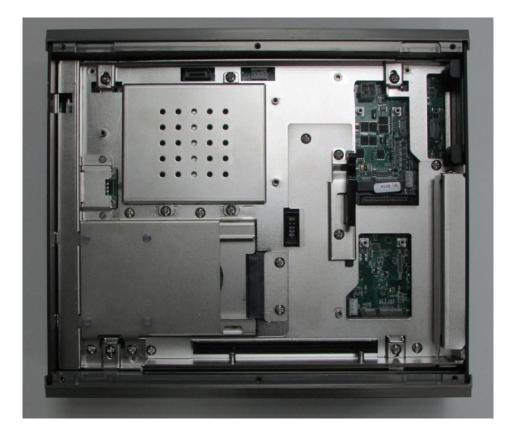
3. Push into the 4 latches as indicated and fasten the 4 screws.
