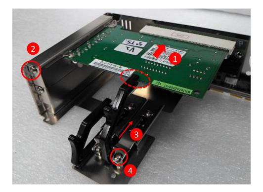
6. Locate the riser card slot on bottom side of system.
