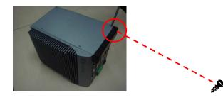
Step 3 Open the top cover and locate the Hard Disk Drives as red marked.
