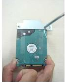
**Step 5** Insert the HDD module into the HDD socket.
