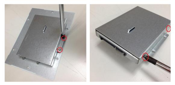
Step 4 Put the HDD bracket on the cover and use 4pcs screws to fix tightly. Takes the
