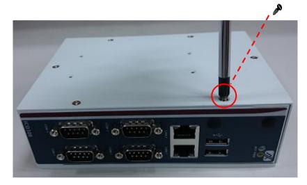
Step 2 Loosen all screws of the cover and remove the cover from the system.
