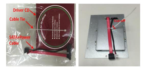
Step 5 Connect SATA+Power HDD cable to the board connector, SATA side first then
