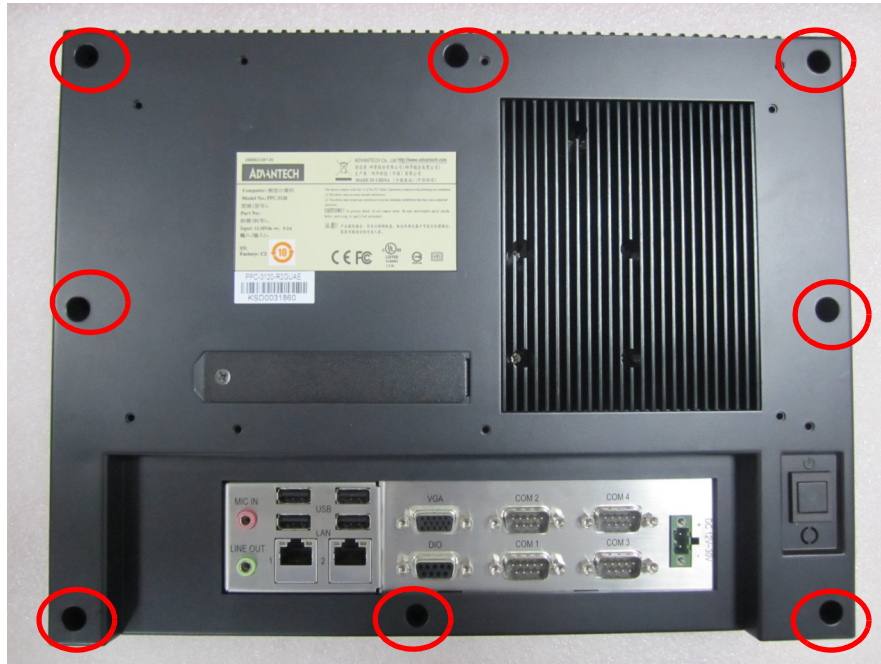
Figure 2.5 Unfastening Screws on Rear Cover
