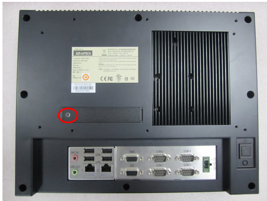
Figure 2.22 Removing Metal Cover
