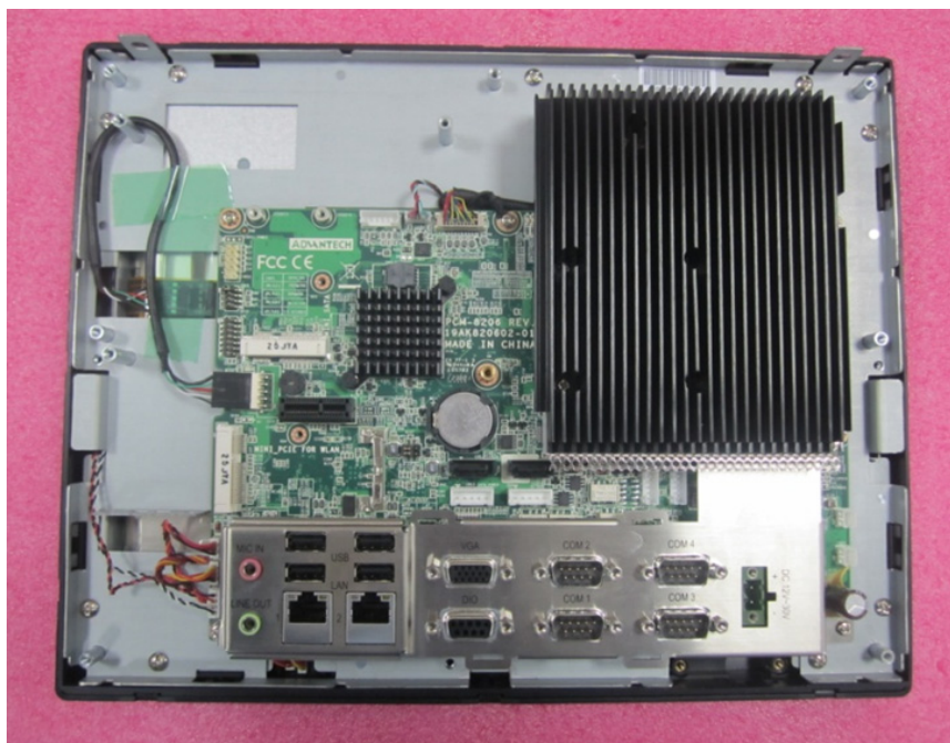
Figure 2.13 Removing HDD Bracket
