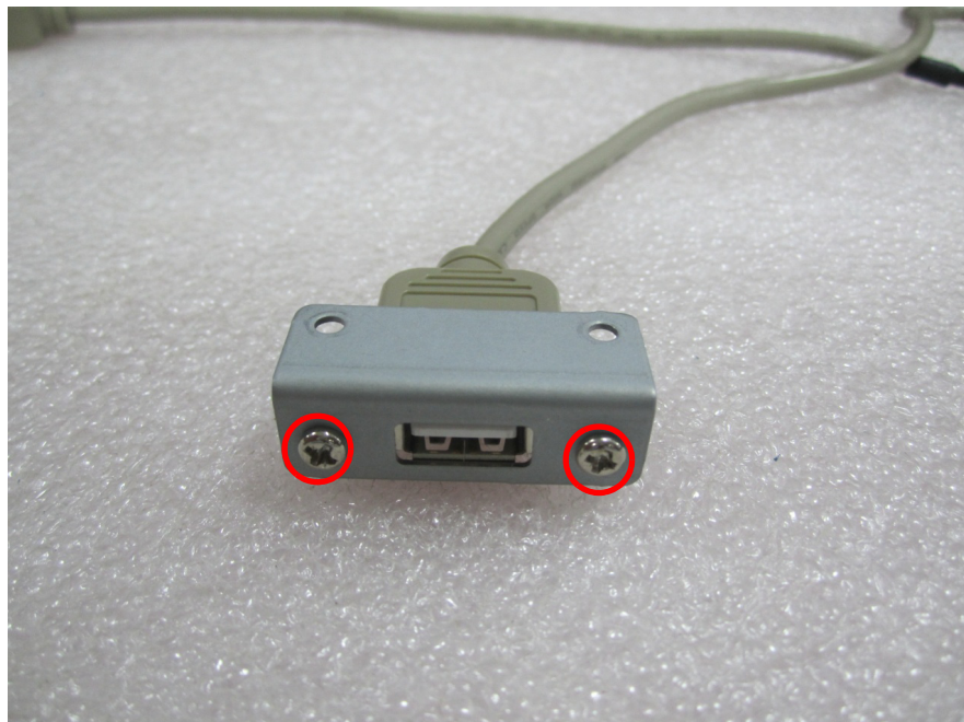
Figure 2.32 Fixing Bracket onto USB Connector
