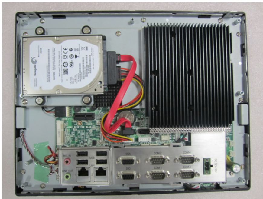
Figure 2.33 Removing Rear Cover
