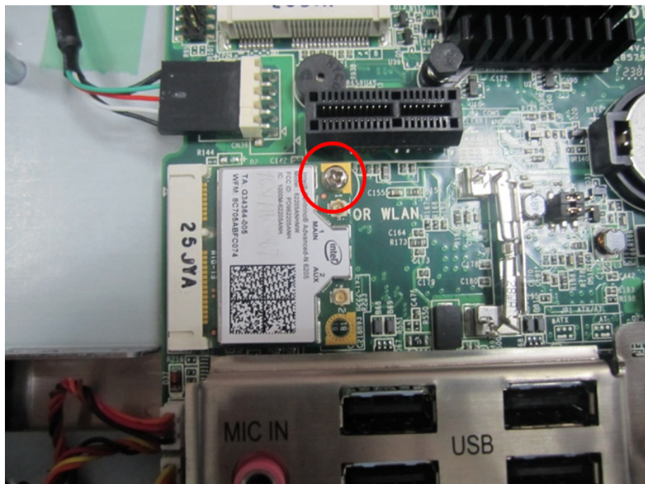
Figure 2.15 Installing Wireless LAN Card
