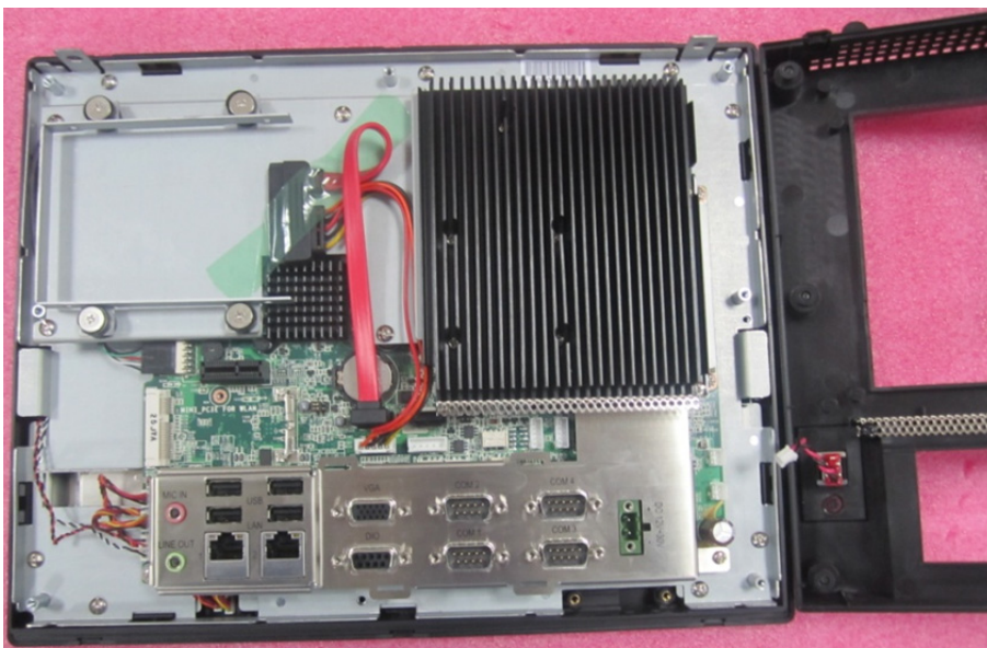
Figure 2.9 Removing Rear Cover
