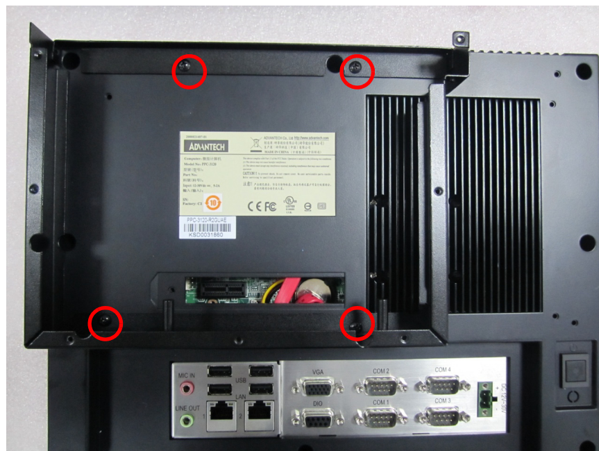
Figure 2.23 Fixing Metal Cover
