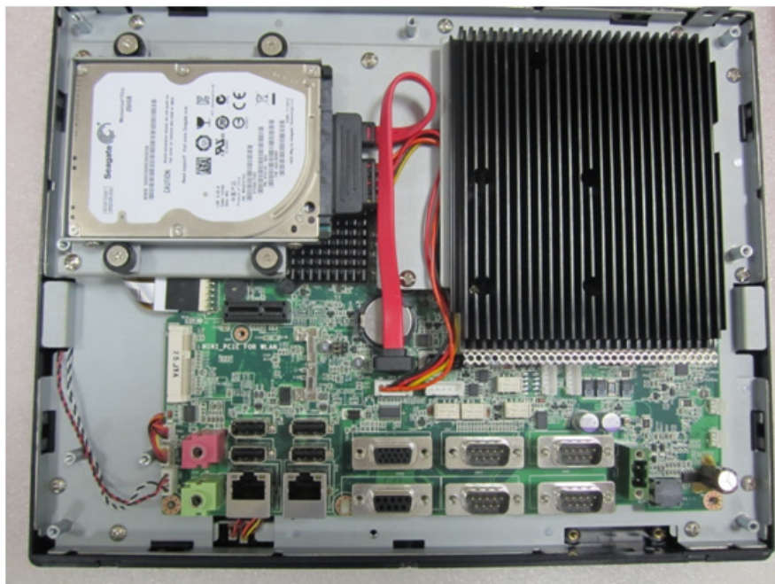
Figure 2.34 Removing IO Shield
