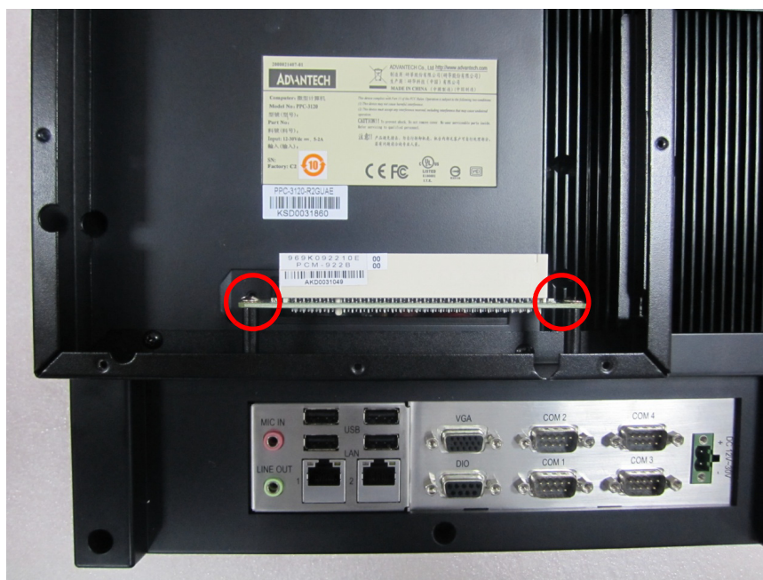
Figure 2.24 Installing Riser Card
