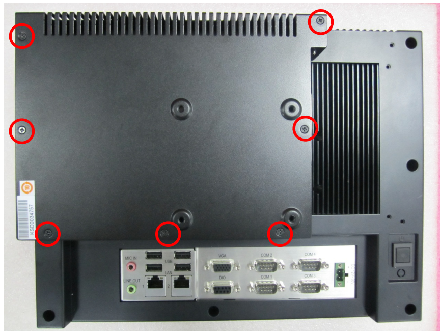
Figure 2.26 Fixing Rear Cover
