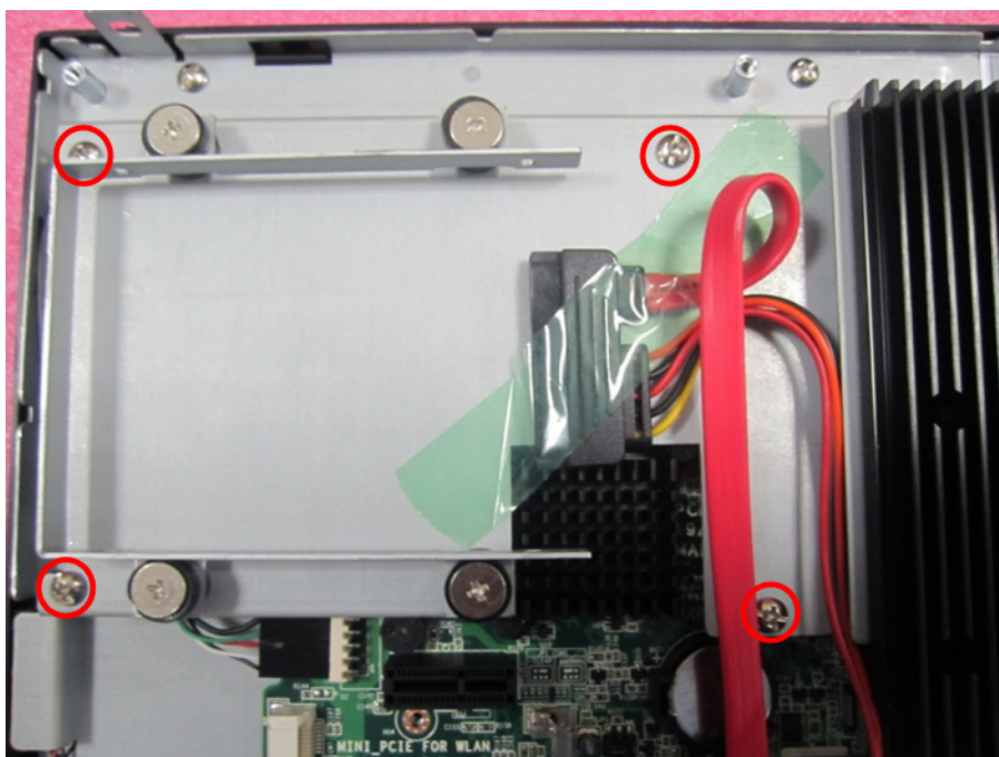
Figure 2.10 Removing HDD Bracket
