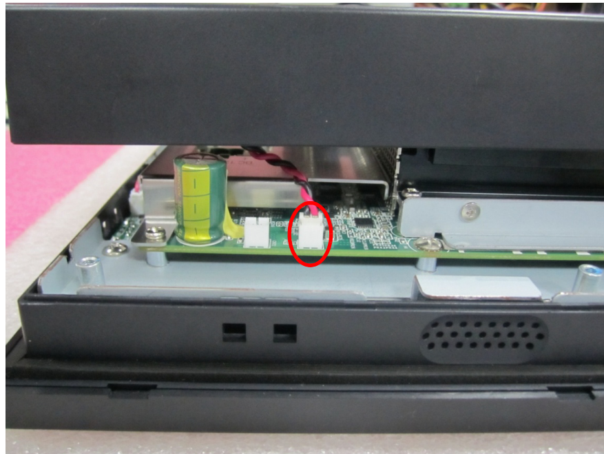
Figure 2.6 Unplugging Switch Wire
