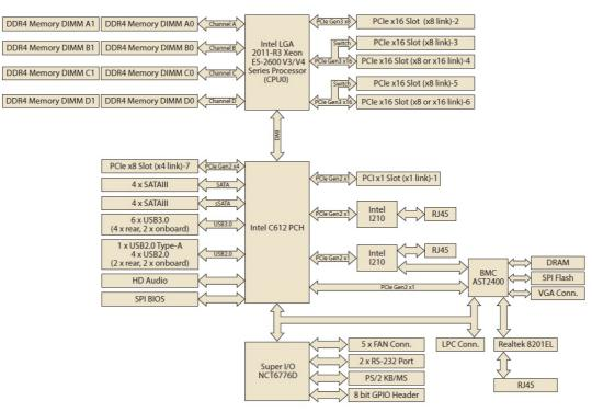
Figure 1.3 Block Diagram
