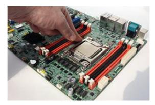
7. Push down both levers and insert them under the retention tabs ensuring the edge of the load plate is fixed securely by both levers.
