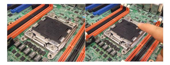
2. Press the other lever and move it sideways slightly until it is also released from the retention tab.
