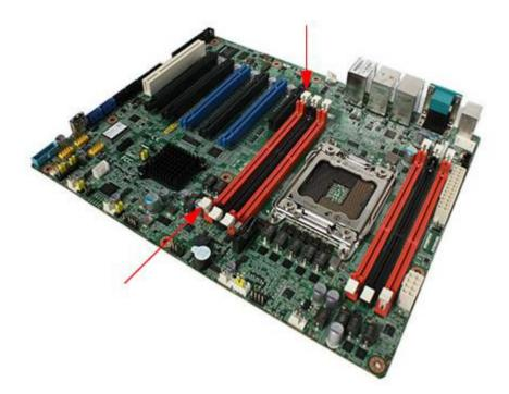
2. Slowly slide the DIMM module along the plastic guides on both ends of the socket,
