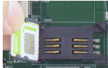
Insert SIM card with pins facing up
