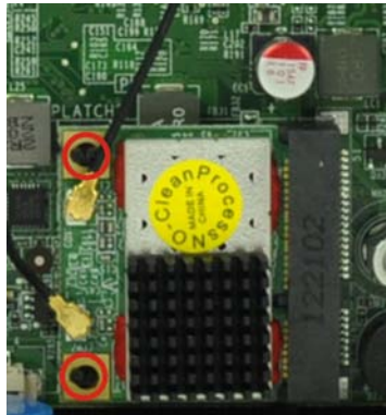
Figure 5-10: Releasing the WLAN Card
