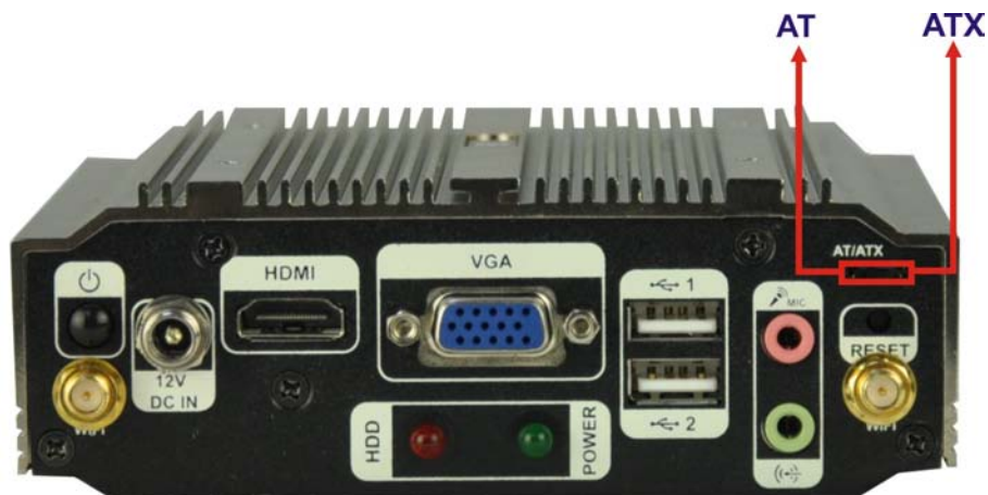
Figure 3-2: AT/ATX Switch Location
