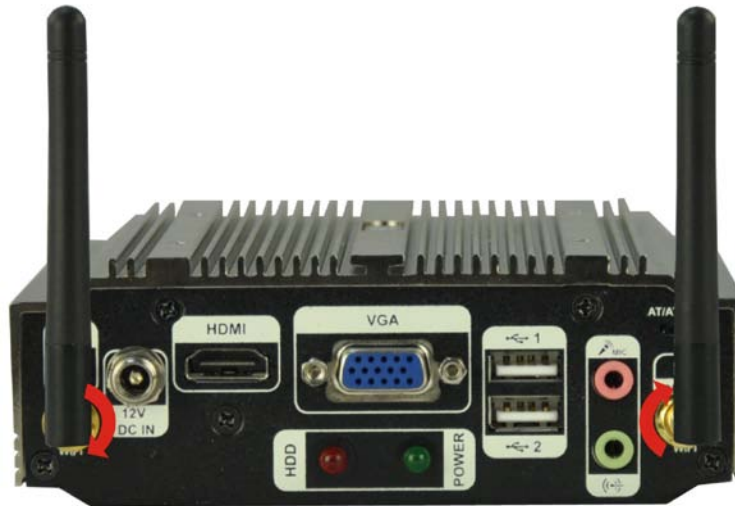
Figure 3-1: Wi-Fi Antenna Installation
