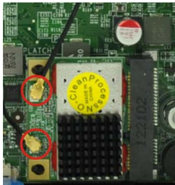
Figure 5-9: Removing the Antennas
