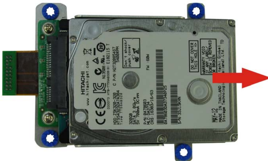
Figure 5-5: Remove the old HDD
