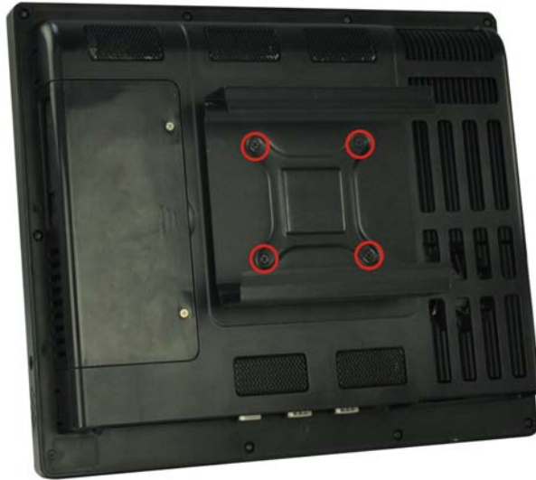
Figure 3–15: Mount Kit Installation
