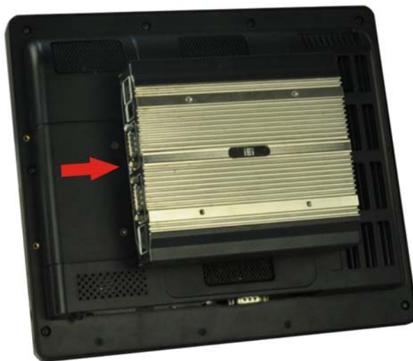
Figure 3-10: Slide the System
