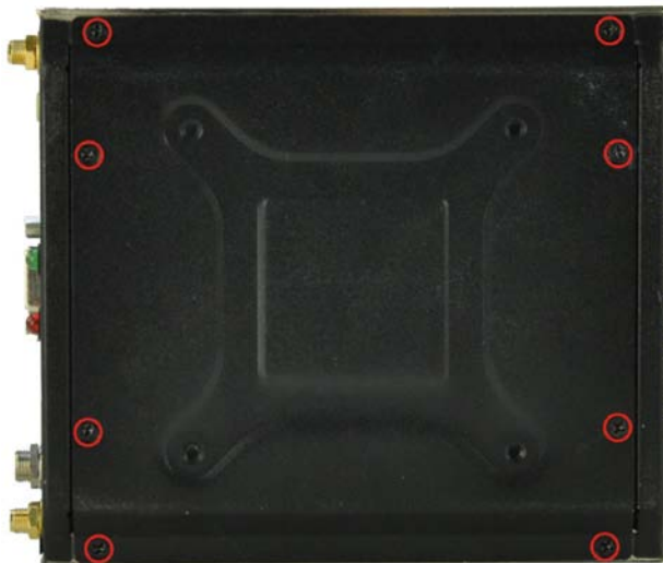
Figure 5-1: Retention Screws Removal
