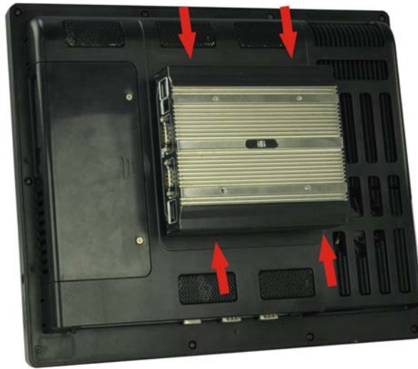
Figure 3-17: Mount Kit Screws
