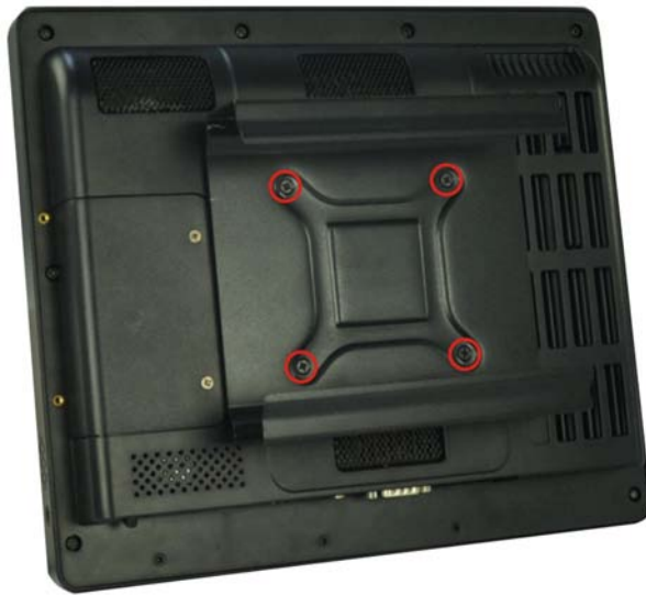
Figure 3-9: Mount Kit Installation
