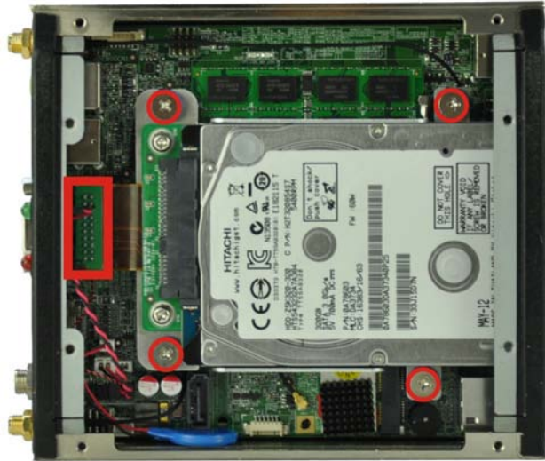
Figure 5-2: HDD Bracket Retention Screws
