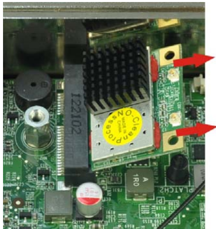
Figure 5-11: Removing the WLAN card
