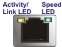
**Figure 3-12: RJ-45 Ethernet Connector**
