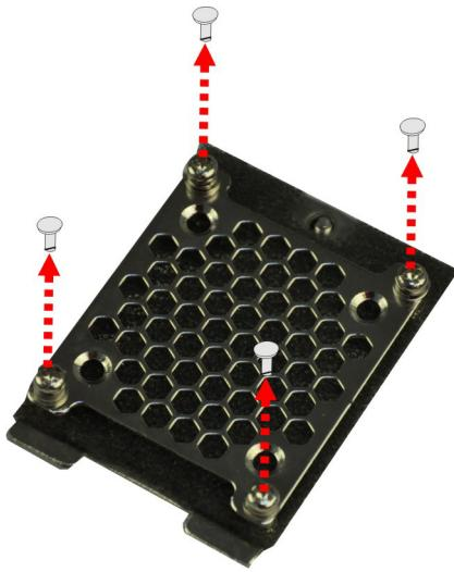
**Figure 3-6: Remove the Fan Bracket from the Cover**
