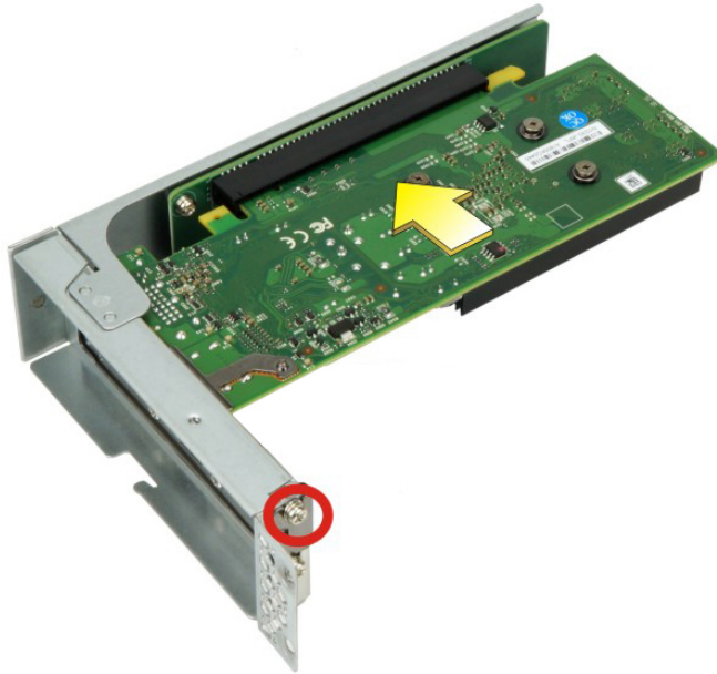
Figure 3-9: PCIe Expansion Card Installation
