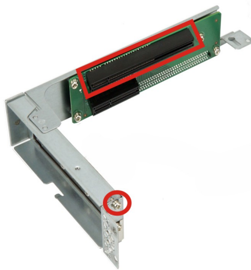
Figure 3-8: Blank Bracket Screw
