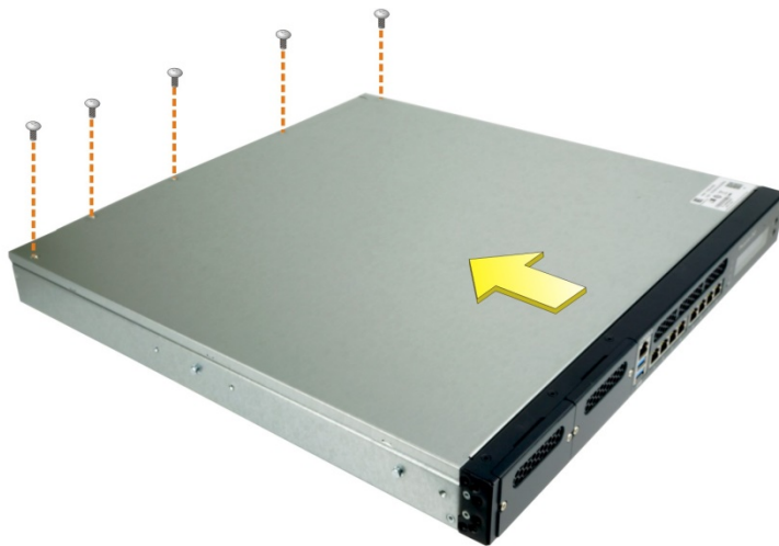
Figure 3-1: Top Cover Removal
