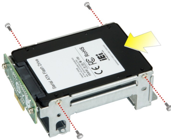
Figure 3-4: Secure HDD to the Bracket
