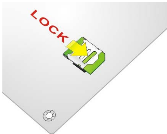
Figure 4-13: Lock SIM Card Slot Cover
