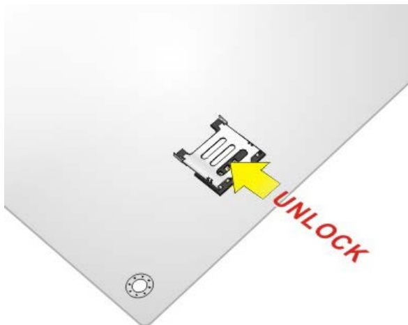
Figure 4-11: Unlock SIM Card Slot Cover
