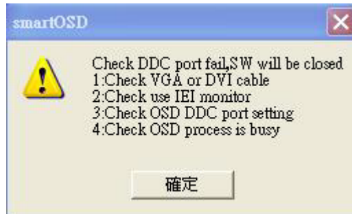
Figure C-18: DDC Port Failure
