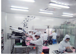
Control room particle measure result: Class 10000
