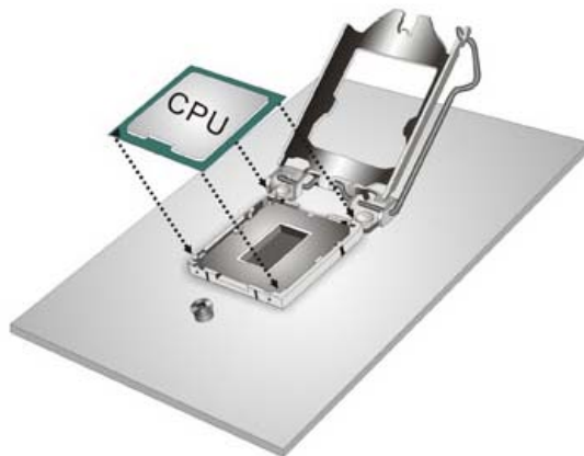
Figure 4-3: Insert the Socket LGA1150 CPU
