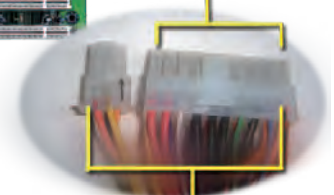
20+4 pin-ATX power connector
