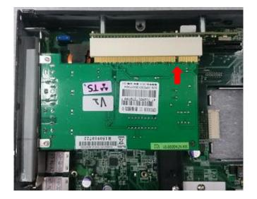
5. Fasten one screw to secure the PCI(e) expansion card.
