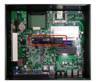
2. Loosen one screw halfway as indicated to have the clamp arm slidable.
