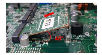
3. Fasten the card with two screws.
