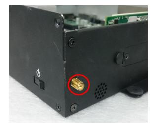
3. Put on the washer and fasten the nut with antenna jack.
