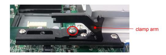
3. Loosen one screw to remove the PCI bracket.
