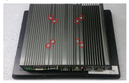
The following picture uses a panel PC (P2000+CV display module) as a demonstration. To attach the panel PC to a VESA stand, please fasten eight screws as indicated to fix it on the stand. (Please refer to section 3.16 in this manual for how to attach PC2000 to CV display module.)
