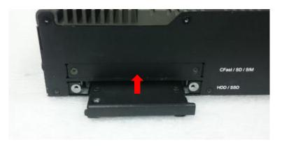
7. Put back HDD bay cover at front panel, and fasten it with two screws.
