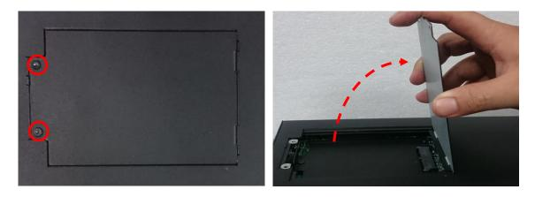
3. Loosen three screws and take the HDD bracket out of HDD compartment.
