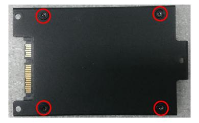
5. Seat the HDD bracket into HDD compartment, and line up the connector of HDD with SATA slot, then push it until HDD is fully connected into slot.
