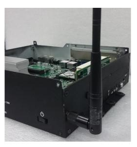
5. Attach the RF connector at another end of the cable onto the card.
