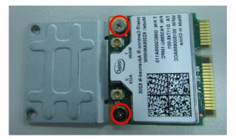
3. Tilt the Mini PCIe card at a 45-degree angle and insert it into the socket until the golden finger connector of the card seated firmly.
