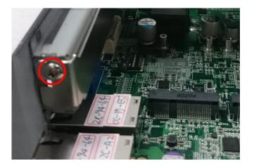
4. Align the notch of golden fingers of PCI(e) card with the expansion slot. Insert the card horizontally, and press the card straight down into the slot until it's seated firmly.
