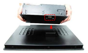
7. Align the mounting holes of P2000 with the screw holes of display module underneath. Then slide the PC2000 carefully as indicated to have P2000 and display module connected together.
