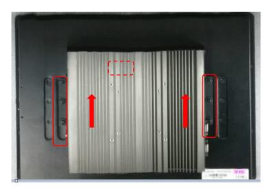
8. Fasten six screws to secure P2000 on the display module.
