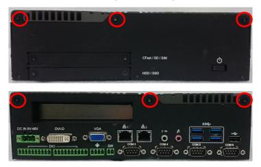
2. Raise the left edge of top cover (1), and raise the other side (2) subsequently to remove it from the chassis.
