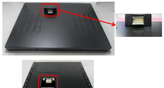
6. Place the P2000 on the display module through its display connector hole as indicated.
