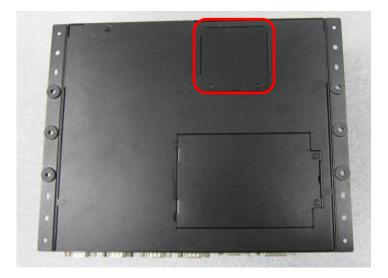
5. Loosen two screws to remove the cover.
