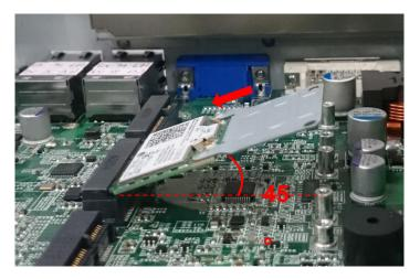
4. Press down the module and use the two screws to fix the module.
