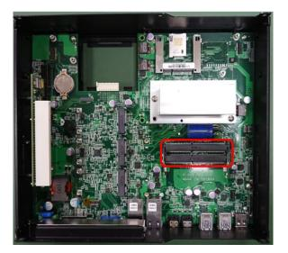
2. Tilt the SODIMM module at a 45-degree angle and insert it to SODIMM socket until the gold-pated connector of module contacted firmly with the socket.
