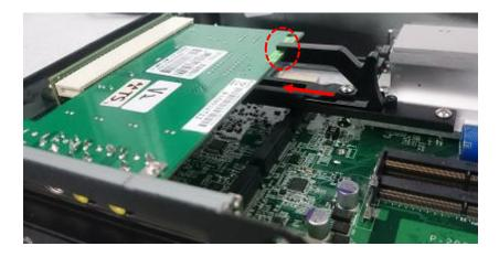
7. Finally, fasten the screw that were previously loosen halfway to fix the retention module.
