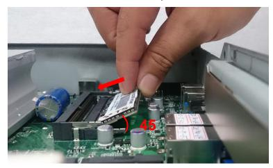
3. Press the module down until its fixed firmly by the two locking latches on each side.
