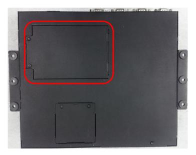
2. Loosen the two screws, then pull the cover to remove it.
