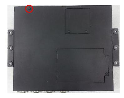
1. Turn over the system to bottom side, and remove one screw.
