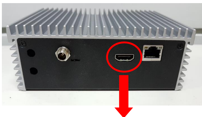
HDMI connector (PICO512-CN15) on rear side
