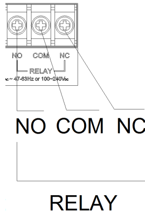
Figure 2.8 Relay output connections
