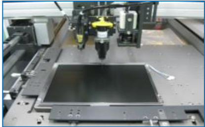
Gluing the gap between frame and panel
