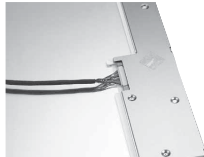
Photo 2 - Plug the LCD side adapter to the applied LCD Panel
