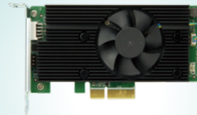
Mustang-V100-MX4 Intel® Movidius™ Myriad™ X MA2485 VPU
